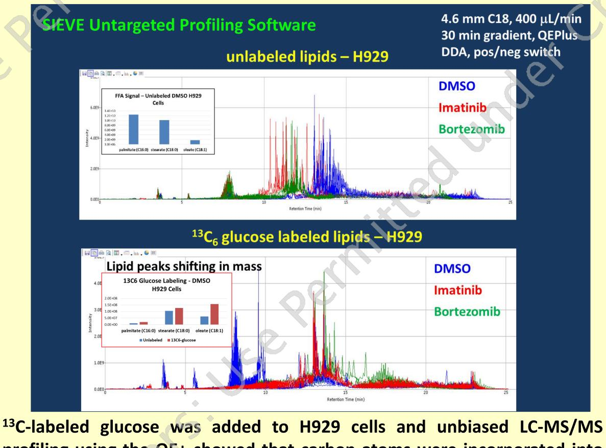
profiling using the QE+ showed that carbon atoms were incorporated into several lipid species based on m/z shifting after lipid extractions.
