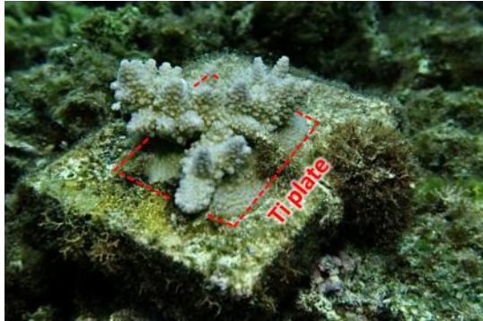
Figure 6. An example of a coral growing on CP-Ti in the offshore (Yoron Island, Kagoshima, Japan). CP-Ti plate was glued on the surface of the mortar base. The fragment of coral was fixed on the CP-Ti plate with SUS304 wire.
