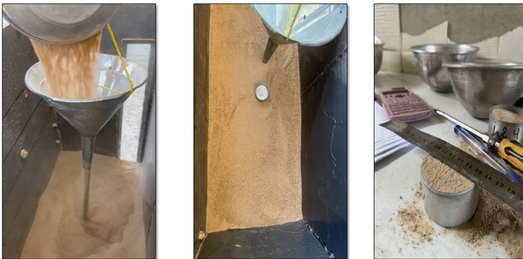
Figure 2. Represents the raining technique.
