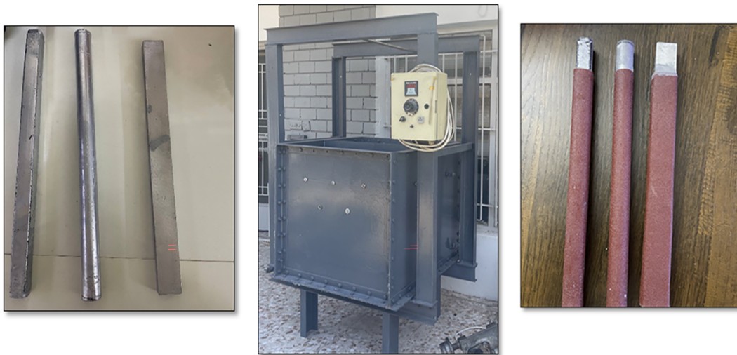
Figure 1. Shows the aluminum pile models with different geometries and a steel laboratory box container.
